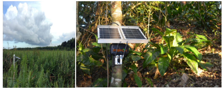
Fig. 1: ARBIMON biodiversity monitoring stations will be the core of a global network. The solar powered stations include an ARBIMON recording device (Android smartphone) with a cellular data plan, which is used to upload recordings in real-time to the ARBIMON II bioacoustics analysis platform. In addition, a companion app uploads status reports on the state of the battery, cellular connectivity and recording collection and upload. Photo: Sieve Analytics.
